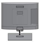
**3** Seat the TV onto stand by pressing the top of the TV slightly.
